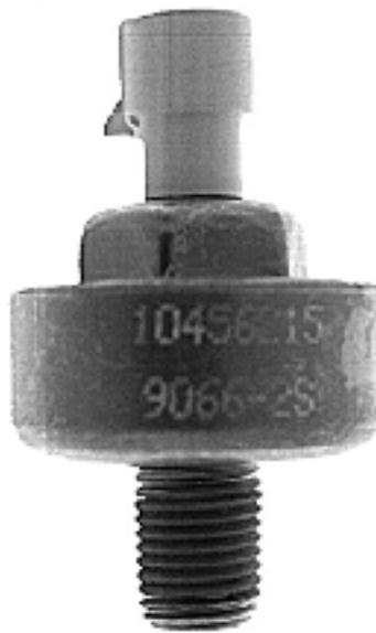
A knock sensor can be used in conjunction with electronic spark control to optimize the ignition advance for the fuel being used. One limiting factor in ignition timing control is 'knocking', which is uncontrolled burning of the fuel in the combustion chamber. This can be affected by intake air temperature, coolant temperature, engine age and condition, air/fuel ratios, air density, altitude and humidity, among others.
