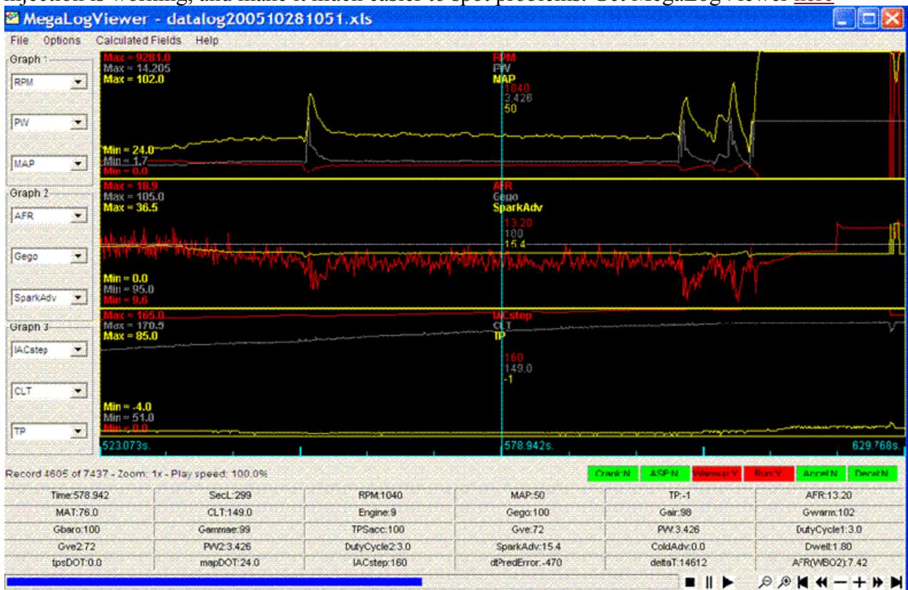
Note that the datalog includes an 'EngineBit' field. This bit will tell you if the engine was accelerating, warming-up, etc., and can be used to sort unsuitable data lines (because O2 correction is not active under acceleration, warm-up, etc.) from the file.
